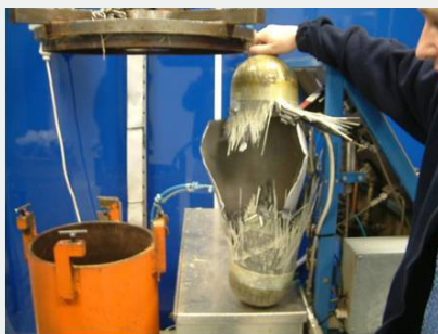
Hydraulic pressure testing dangers
